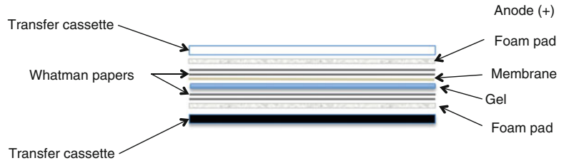
Fig. 2 Schematic representation of the sandwich assembly for the Western blot
